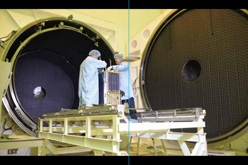
The Houwteq thermal test facilities include a large thermal vacuum chamber and a medium thermal vacuum chamber.
