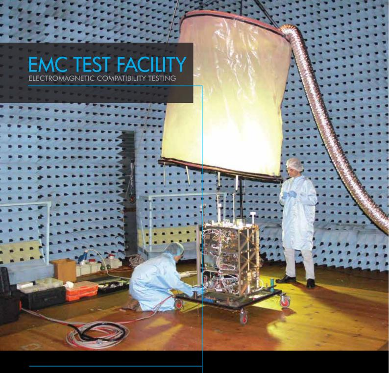
The EMC Test Facility at Houwteq provides Electromagnetic Compatibility (EMC) testing services to the commercial, aerospace and defence industries.
